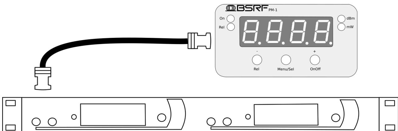
Illustration 3: Connecting PM-1 to an IEM TX(BNC)
