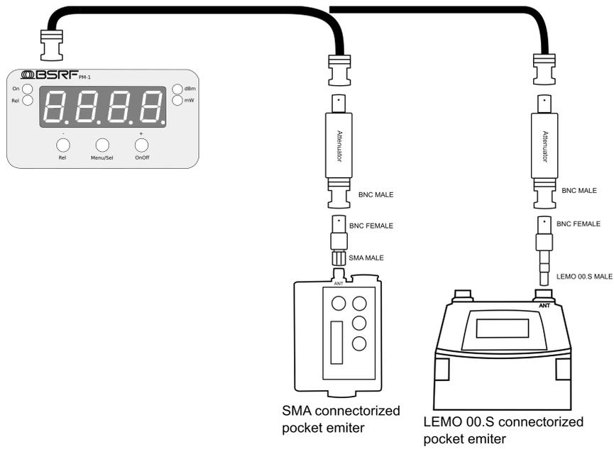
*Illustration 5: Adding an attenuator to reduce SWR effects*
